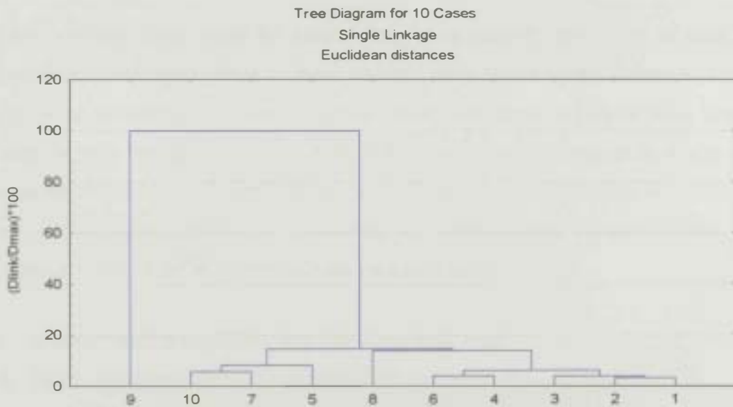
Figure 4.10 Cluster analysis for heavy metals (Cu, Ni, Pb, Zn, Cr) in the surface sediments along Dubai Creek during 1999
